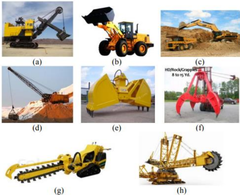
Figure 1. Standard land excavating equipment. (a) Power shovel. (b) Front-end loader. (c) Backhoe. (d) Dragline. (e) Clamshell. (f) Grapples. (g) Trencher. (h) Continuous bucket excavator
